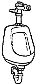
URINAL WITH A P-TRAP CONNECTION
